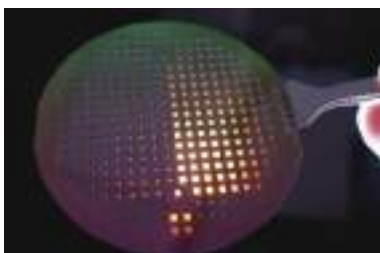
One and four quadrant 10 micron thick silicon diode for synchrotron beam monitoring
