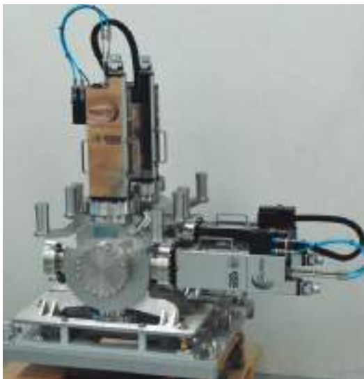
Emittance Meter Unit for MYRRHA project (ESS-Bilbao & SCK CEN)
