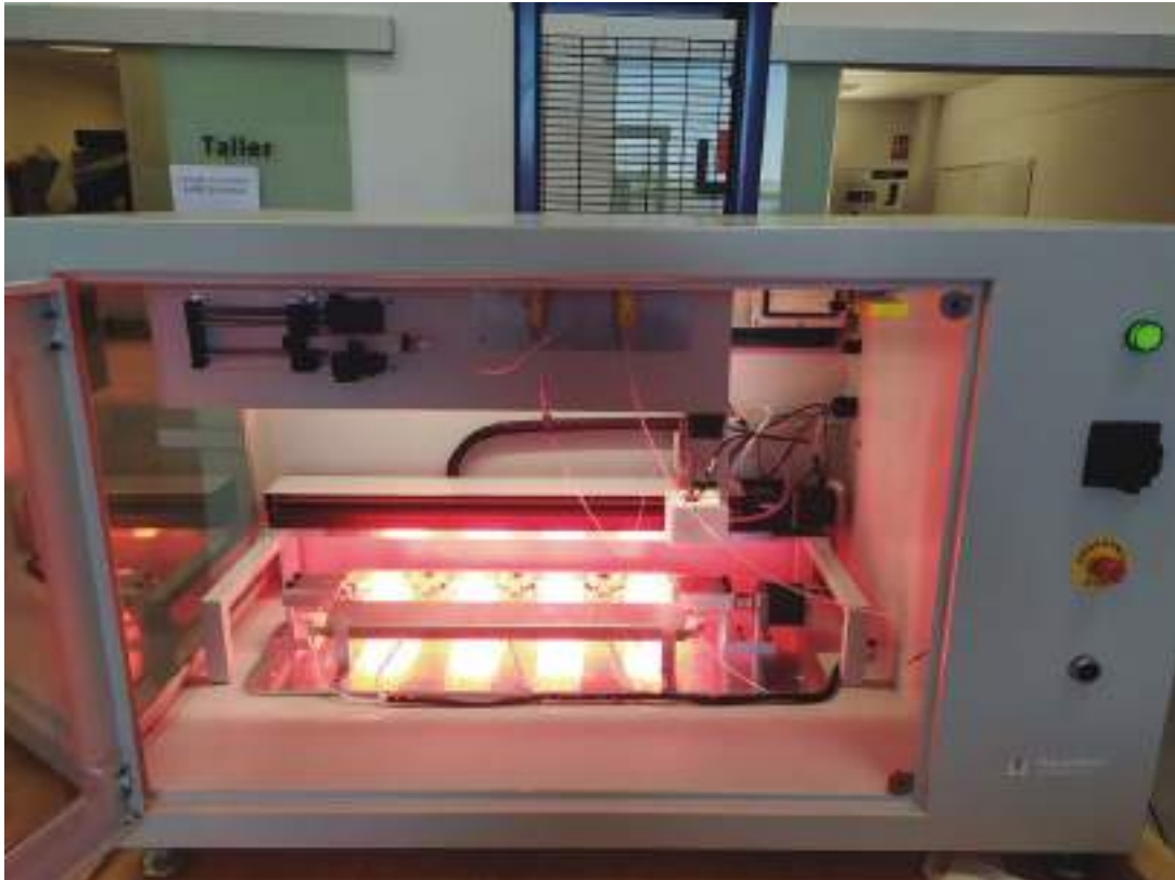
Customized ultrasonic spray for coating tubes
