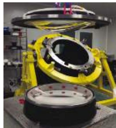
WHT WEAVE Optical Corrector System Integration
