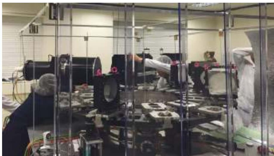
MEGARA spectrograph for the GTC 10m telescope during the assembly at laboratory in Universidad Complutense (customer UCM, Madrid)
