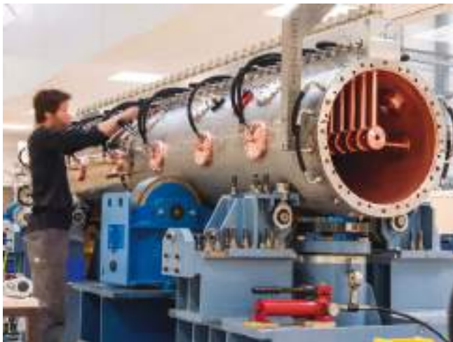
CERN dtl tank
