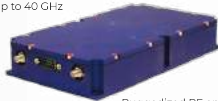
Ruggedized RF optical delay line
