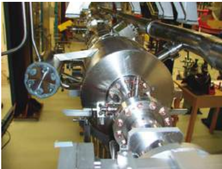
[CIEMAT] Set of superconducting magnets for main lineal accelerator of European XFEL, 2011-2015
