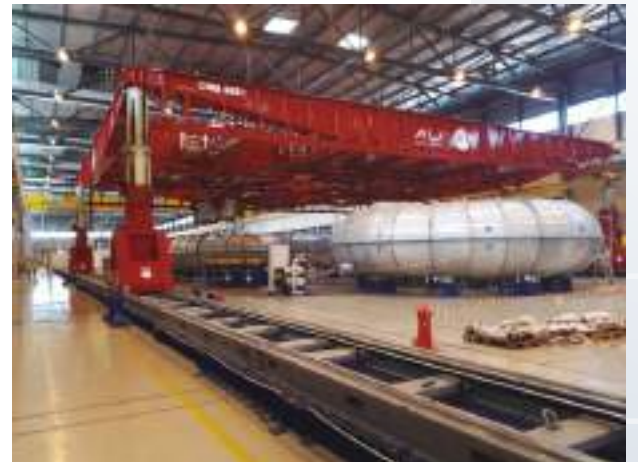
Lifting gantry for the main coils in the ITER project
