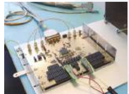
Testing a FPGA based PCB to test camera CMOS sensors under a vacuum environment
