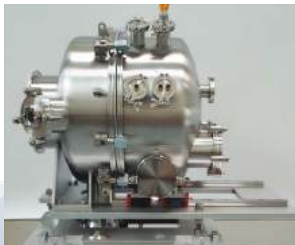
Vacuum Chamber with Temperature Control System form -150° to 200° for CNA
