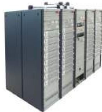
350kW liquid-cooled SSPA for CERN
