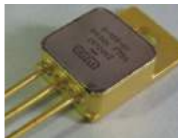
Pacakaged SiC blocking diode
