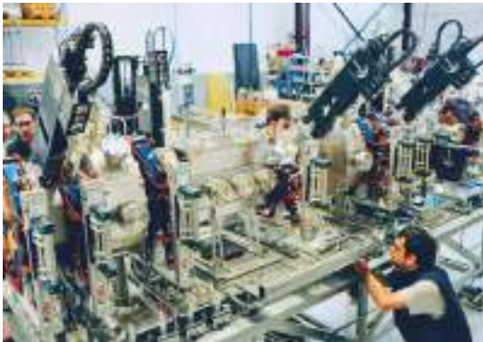
MEBT Assembly at ESS Bilbao premises
