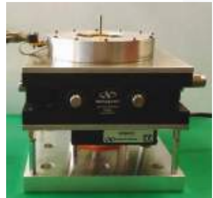
LRPS Low Resolution Angular Sensor (10-bits) for harsh environments (radiation and extreme temperatures)
