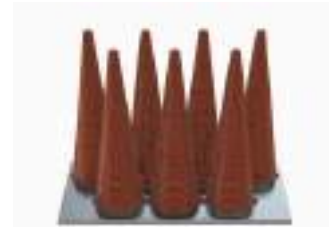
UWB Feed Array cluster for future radiometers
