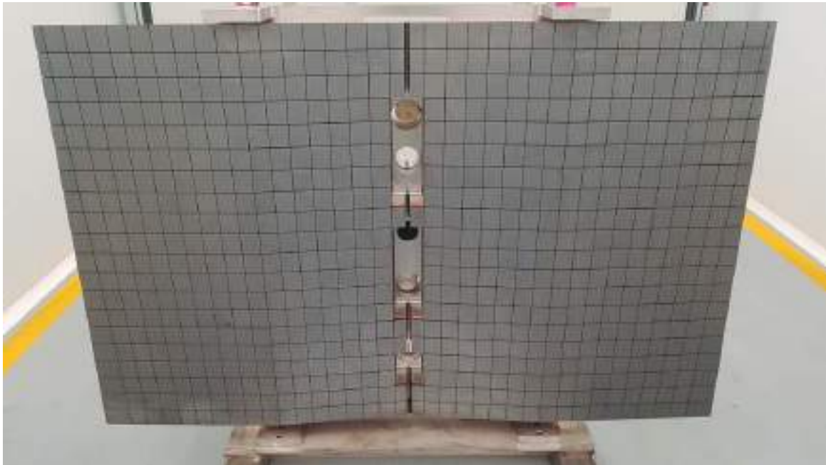
Finished First Wall Panel Semi Prototype
