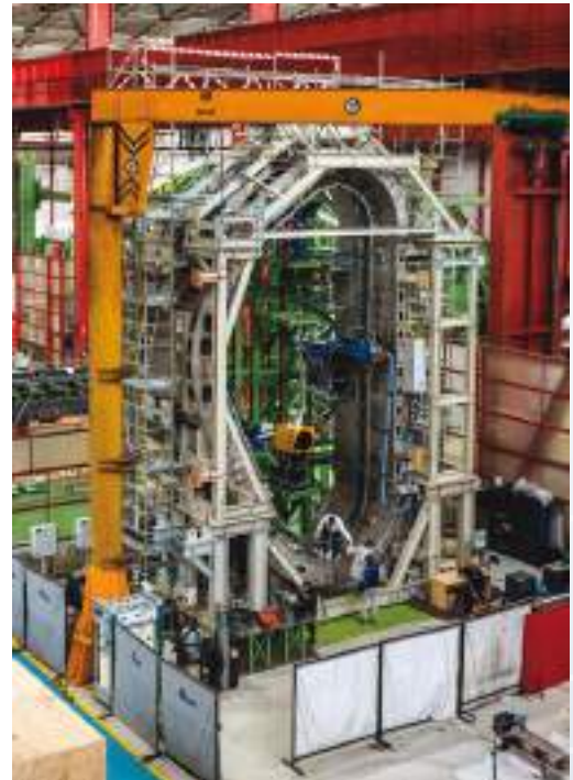
ITER vacuum vessel welding mockup
