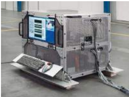
EGSE for Sampling Tool Mechanism
