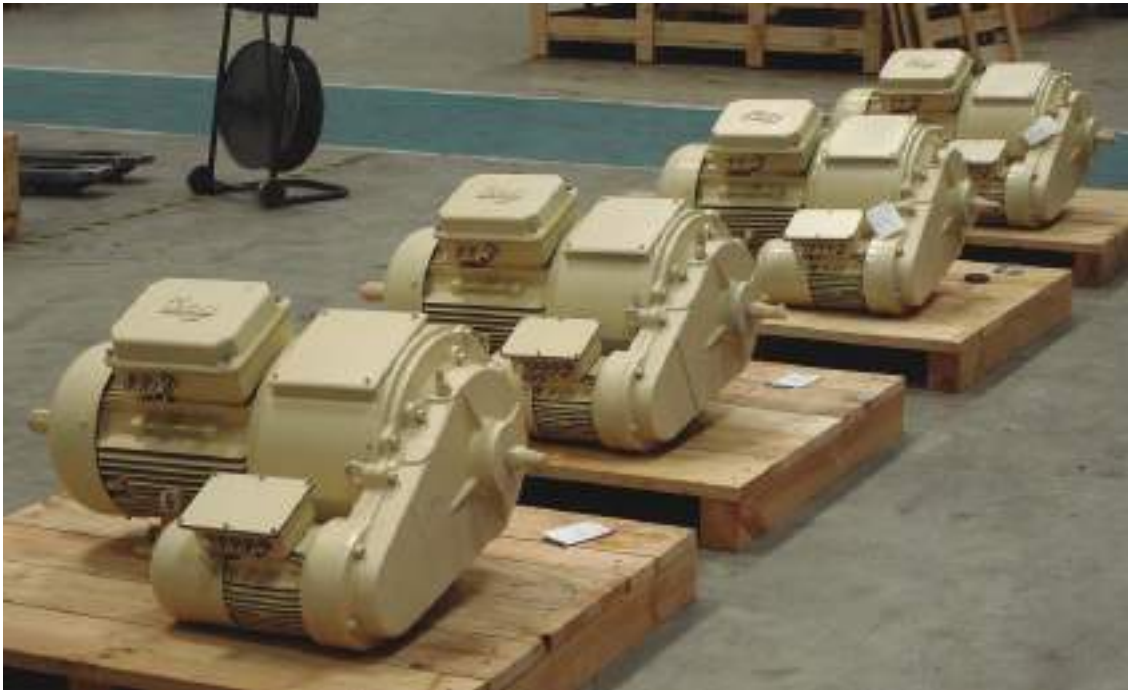
A set of OBEKI microspeed brake-motors manufactured for a French nuclear power plant
