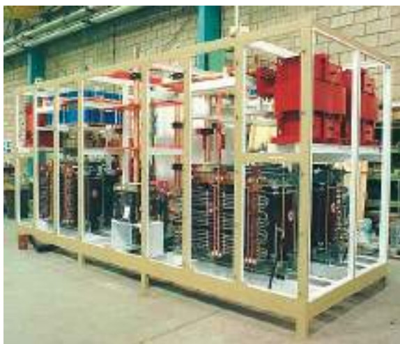
DC Power Supply for CERN
