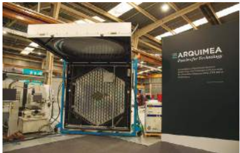
ARQUIMEA project - cameras for Cherenkov North Observatory
