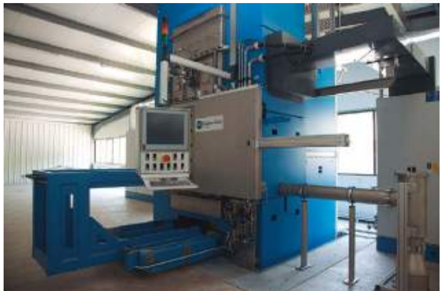
Large scale Spark Plasma Sintering (SPS)
