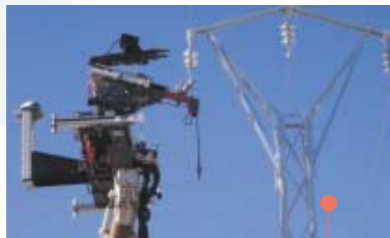
Technological exhibition on occasion of the NPC and HLG meetings of Málaga: Robot for live line maintenance in electrical networks.
