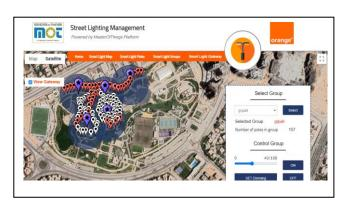
each pole or group of poles and provides status information on the lamp or faults of each pole.
