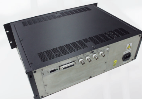
Low Noise Transimpedance Amplifier for fusion diagnostics at JET. 4 channel card in a up to 16 channel crate
