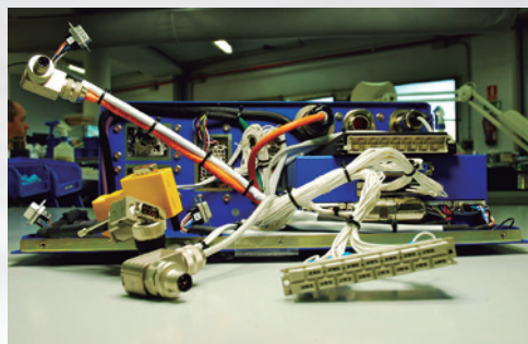
Internal cabling for racks and boxes
