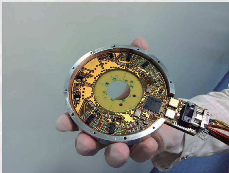
16-bit contactless angular sensor for harsh environments
