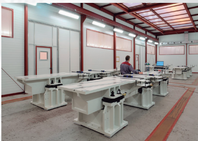
Support structures for the Storage Ring of the SESAME Synchrotron in Jordan
