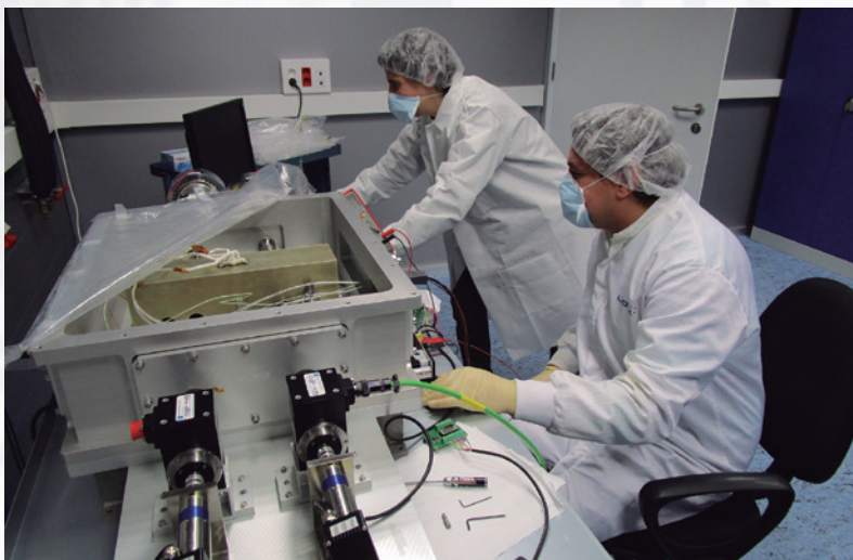
Hot Temperature & Vacuum Chamber used for ITER Optical Samples thermal characterization (250°C)
