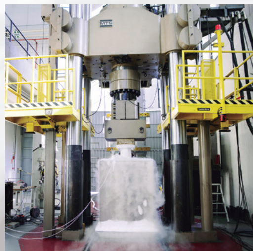
ITER Project - Mechanical Tests on Intercoil Structures at cryogenic temperatures
