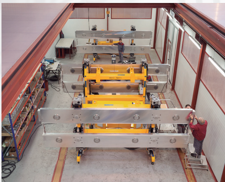
Manufacture, assembly, alignment, commissioning and supply of 40 Insertion Devices Support Systems for the XFEL Project in Hamburg
