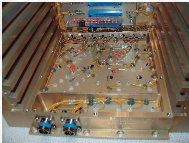
Harness and backplane for satellite power distribution and data links
