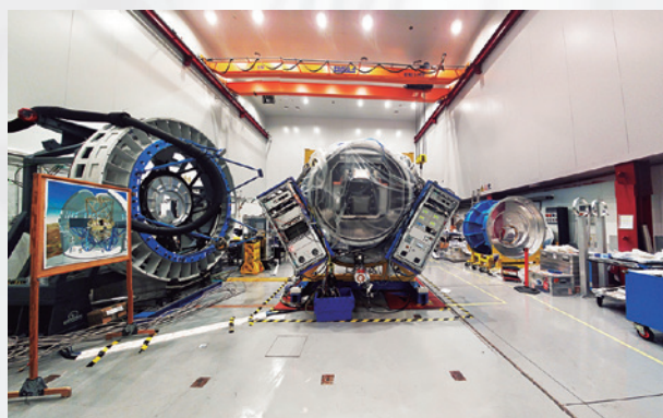
Integration in the AIV room (Assembly, Integration, and Verification of large instruments) of EMIR, a wide-field camera and multi-object spectrograph in the near infrared, designed and built by the IAC for the Gran Telescopio CANARIAS (GTC) at the Roque de los Muchachos Observatory (La Palma, Canary Islands, Spain). © Pablo López /IAC.
