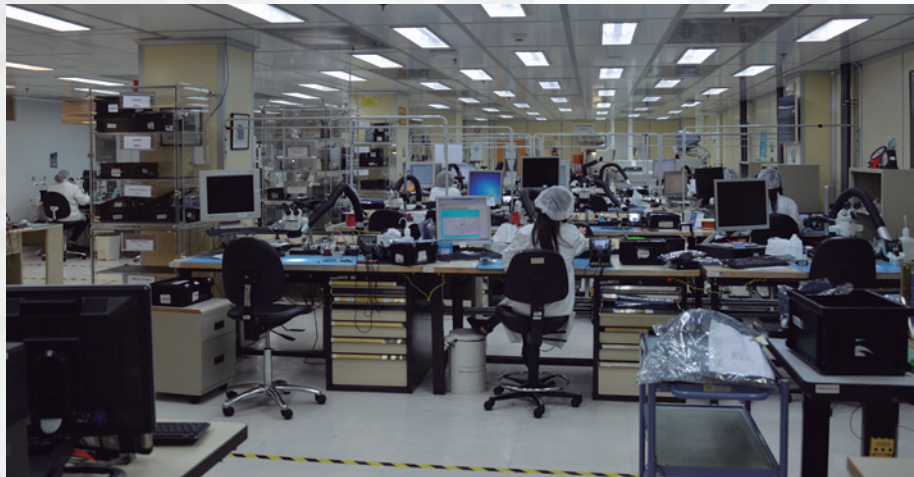
Thales Alenia Space España has a complete 1700m 2 ISO 8 cleanroom for manufacturing and test
