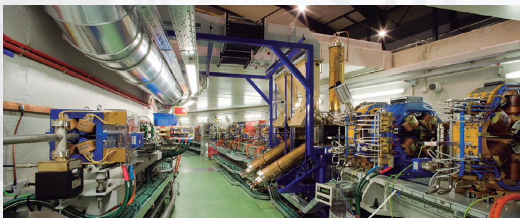
Optical hutch of the XALOC beamline, devoted to macromolecular crystallography
