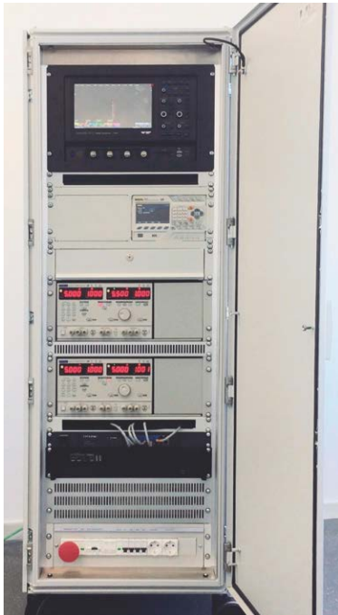
RACK Electrical Ground Support Equipment for testing scientific equipment IR and UV cameras
