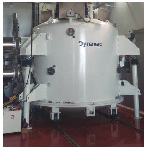
The OAJ vacuum chamber for aluminizing mirrors of up to 3m diameter
