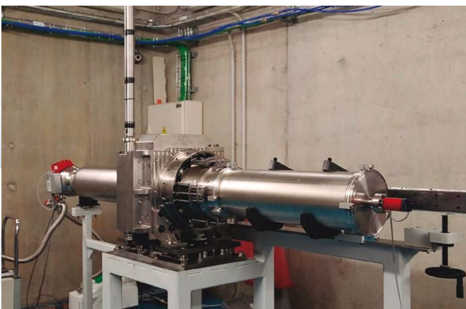
Remote Clamp (ESS) vacuum + remote handling
