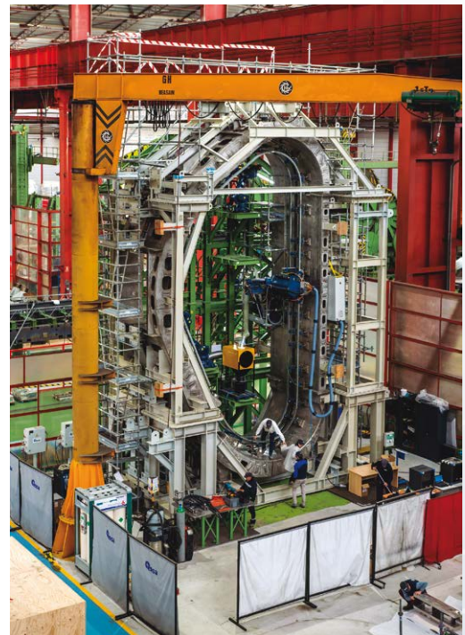
ITER vacuum vessel welding mockup
