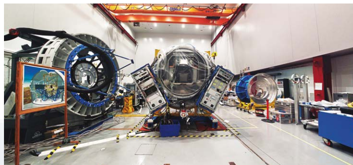
Integration in the AIV room of EMIR, a wide-field camera and multi-object spectrograph in the near infrared, designed and built by the IAC for the Gran Telescopio CANARIAS. © Pablo López /IAC.
