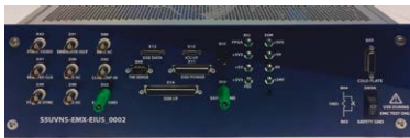
Detail of rack unit for testing charge Coupled Devices for ultraviolet cameras
