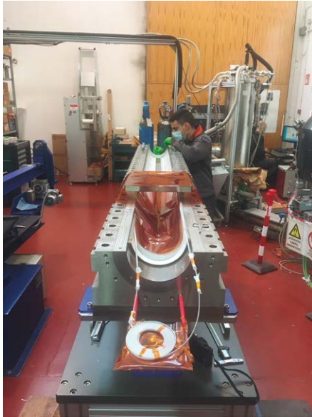
Binding Process of the MCBXFA magnet for the HL-LHC
